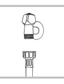
2. Connect the inlet hose by screwing it to a cold water tap using a 3/4 gas threaded connection *(see figure)*.
